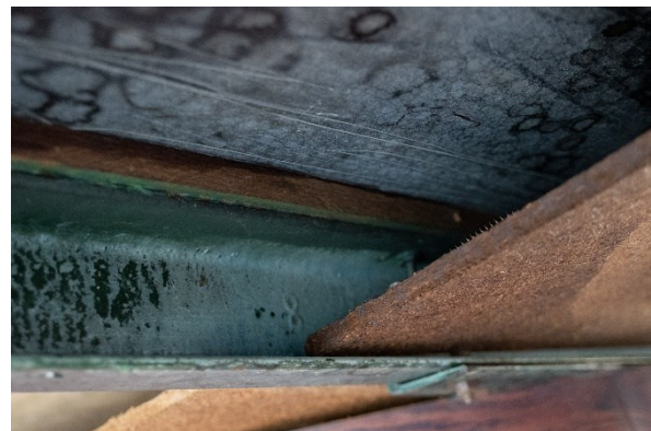
Figure 44: Charring of Table Components
