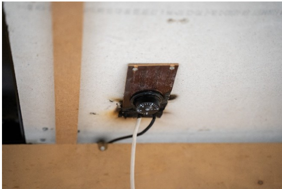
Figure 48: Heating Element in Billiard Table (left) and Radiant Flux Measurement Device (right)
