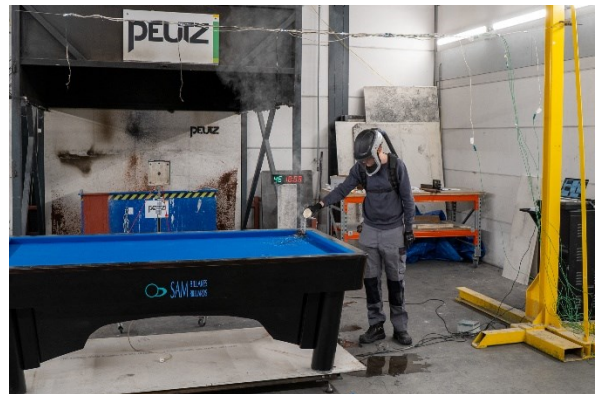
Figure 46: 3 rd Attempt to Bring Table 2 into Flames (left) and Taking out Table Fire 2 with a Cup of Water (right)
