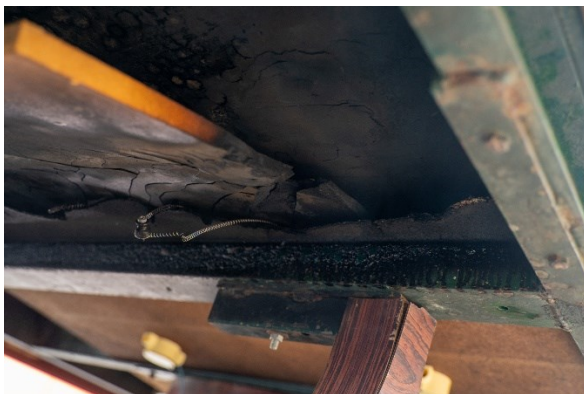
Figure 44: Charring of Table Components
