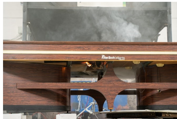
Figure 41: Smoke Beginning to Form (right) and Fire Inside the Table (left)
