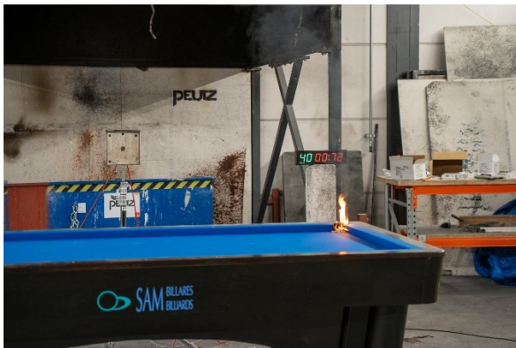
Figure 46: 3 rd Attempt to Bring Table 2 into Flames (left) and Taking out Table Fire 2 with a Cup of Water (right)
