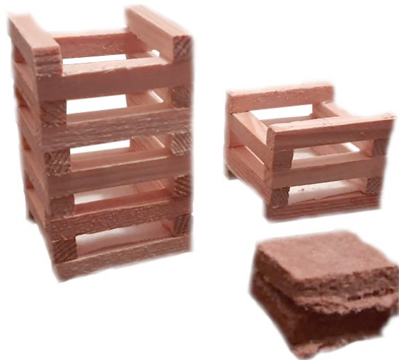
Figure 6: Wooden Cribs and Starting Block used for Starting the Fires
