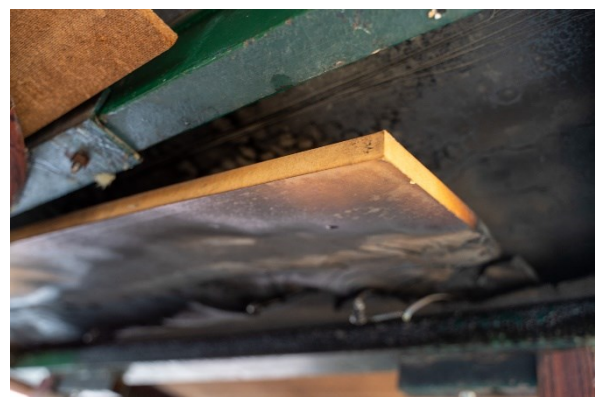
Figure 43: Material Loss of Table (left) and Charring of Wooden Components (right)
