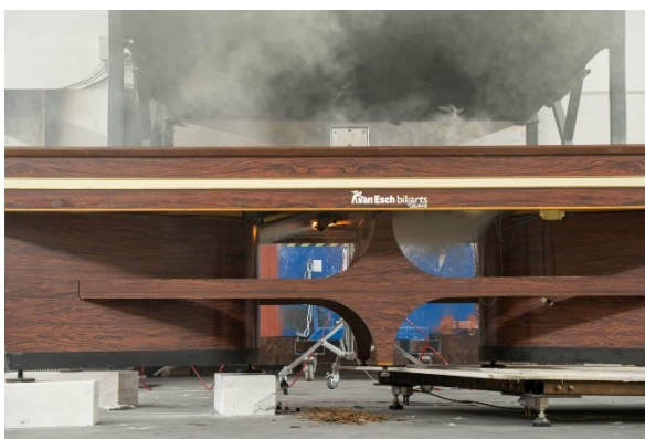
Figure 43: Material Loss of Table (left) and Charring of Wooden Components (right)
