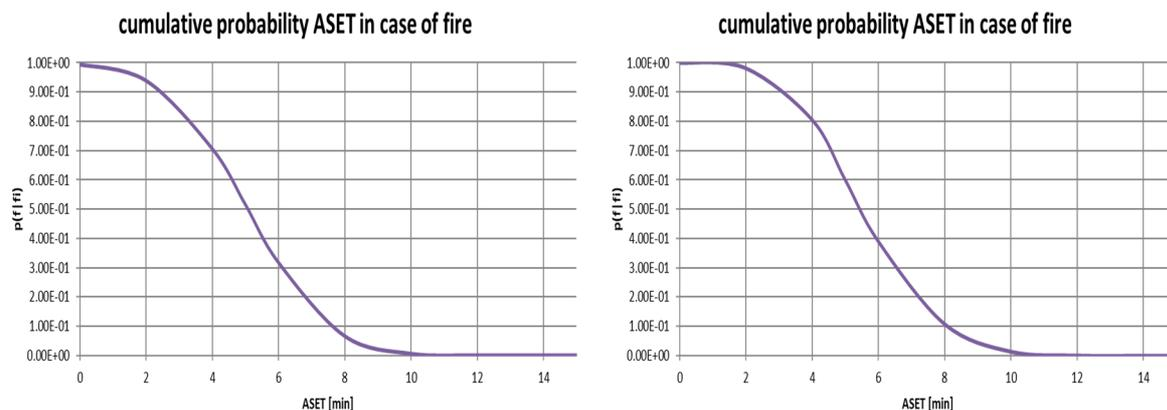
**Figure 8: Cumulative probability distribution ASET in the corridor, criterion visibility (left: non-sprinklered reference situation; right: sprinklered situation)**
