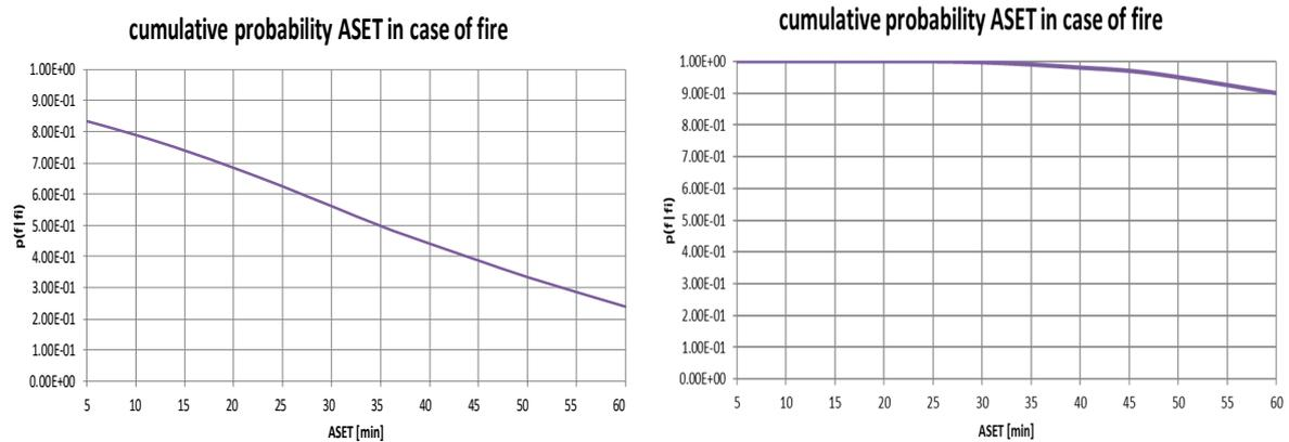
**Figure 10: Cumulative probability distribution ASET in the corridor, criterion CO-dose, after opening of the fire compartment (5 minutes) (Left: non-sprinklered reference situation; Right: sprinklered situation)**
