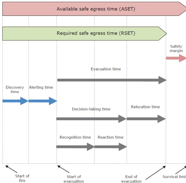
**Figure 1: Safe evacuation is possible if  $ASET > RSET$ . The safety margin is the difference between ASET and RSET (Hagen et al, 2017)**
