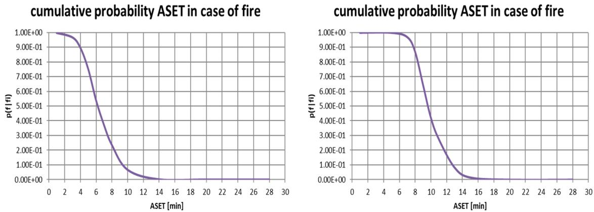
**Figure 7: Cumulative probability distribution ASET in the large compartment with low ceiling, criterion visibility > 5 m (left: non-sprinklered reference situation; right: sprinklered situation)**
