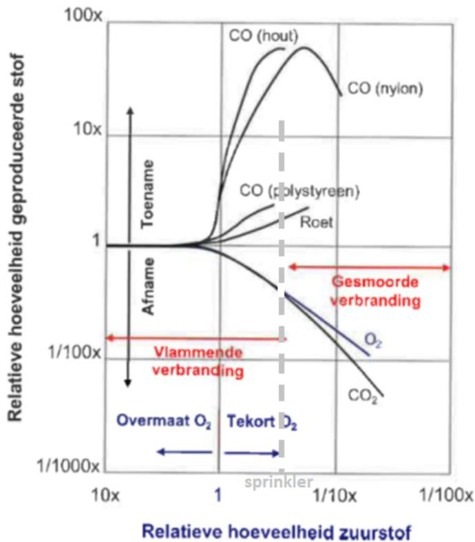
**Figure 4: Production of soot and CO, depending of the degree of smothering. The dashed grey line indicates the local smothering of the sprinkler, whereby the soot yield is increased by a factor 2 and the CO yield by a factor of 10 (Quintière, 1998).**
