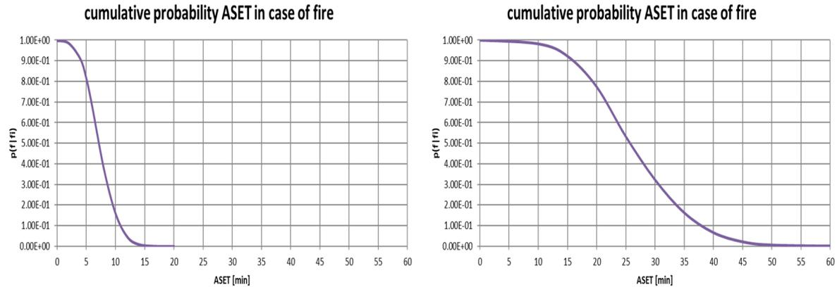
**Figure 11: Cumulative probability distribution ASET in the fire compartment, criterion CO-dose (Left: non-sprinklered reference situation; Right: sprinklered situation)**
