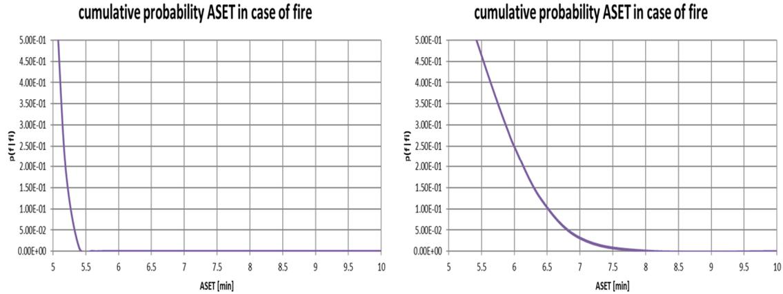
**Figure 9: Cumulative probability distribution ASET in the corridor, criterion visibility, after opening the door of the fire compartment (5 minutes) (left: non-sprinklered reference situation; right: sprinklered situation)**
