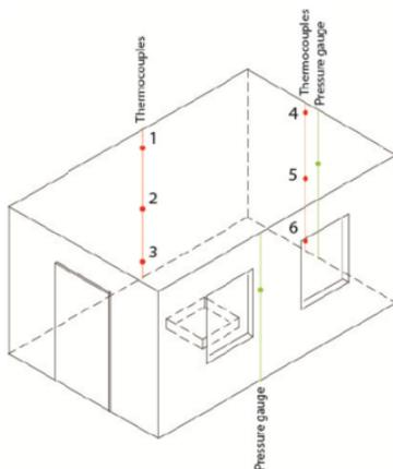
Figure: Experimental setup in a single room
