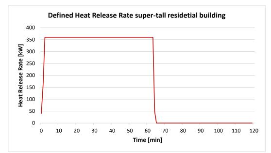
Figure 5-3. Defined Heat Release Rate in a sprinklered compartment of the super-tall residential building.
