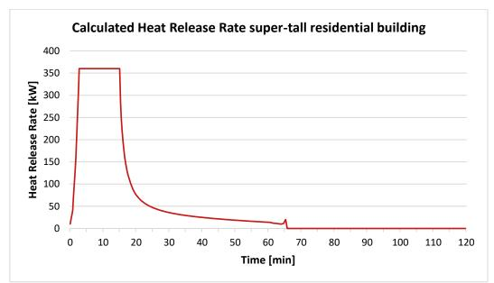
*Figure 5-4. Calculated Heat Release Rate in a sprinklered compartment of the super-tall residential building.*
