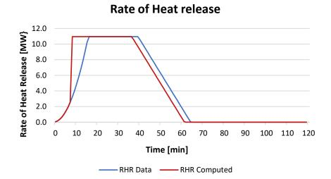
Figure 2-4. Rate of Heat Release (RHR) of natural fire according to Annex E of NEN-EN 1991-1-2/NB, used in the Ozone model.
