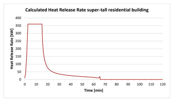
Figure 9-6. Calculated Heat Release Rate in a sprinklered compartment of the super-tall residential building.
