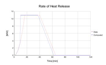
Figure 2. RHR Data and Computed Max: 10.95MW At:10.00 min
