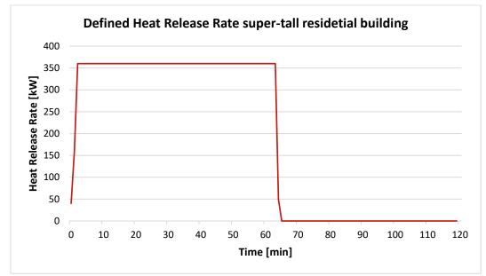
Figure 9-5. Defined Heat Release Rate in a sprinklered compartment of the super-tall residential building.
