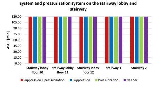
Figure 5-15. ASET overview and the effect of a suppression system and pressurization system on the stairway lobby and stairway.
