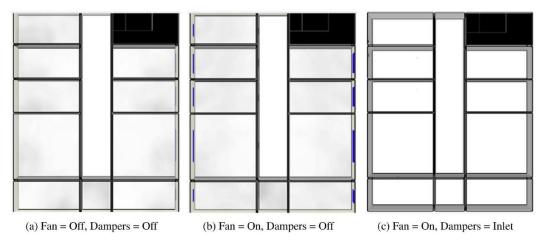
Figure 5-4. Visualization of smoke concentration 170 s after ignition [10]
