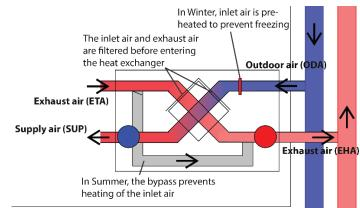
Figure 6-4. Heat recovery ventilation (HRV) unit schematically explained
