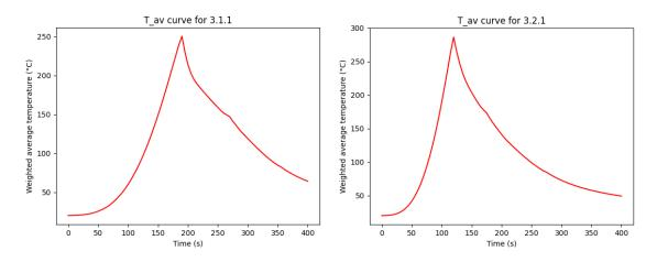
Figure 5-8. Weighted average temperature for fire scenario 3.1.1 where  $t_g = 300 \text{ s}$  (left) and 3.2.1 where  $t_g = 150 \text{ s}$  (right)
