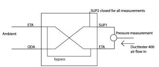
Figure 6-5. Schematic overview of the test set-up
