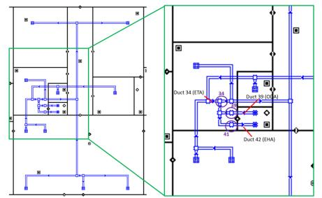
Figure 6-9. Indication of duct segments 34, 39 and 42, and junctions 34, 39 and 41 on the floor plan of apartment 4/A2
