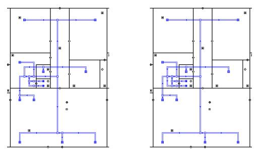
Figure 6-8. CONTAM geometry of apartment 4/A2 without (left) and with (right) modelled bypass
