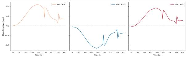
Figure 6-14. Mass flow rates for ducts 34, 39 and 42 when  $t_a = 300$  s
