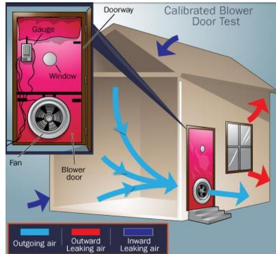
Figure 1 - Measurement setup Blower Door Test, source: (RedPoint LLC, 2017)
