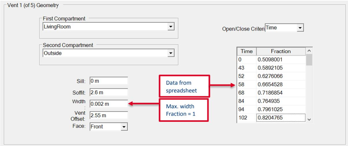
Figure 10 - Changing the opened fraction of openings in CFAST
