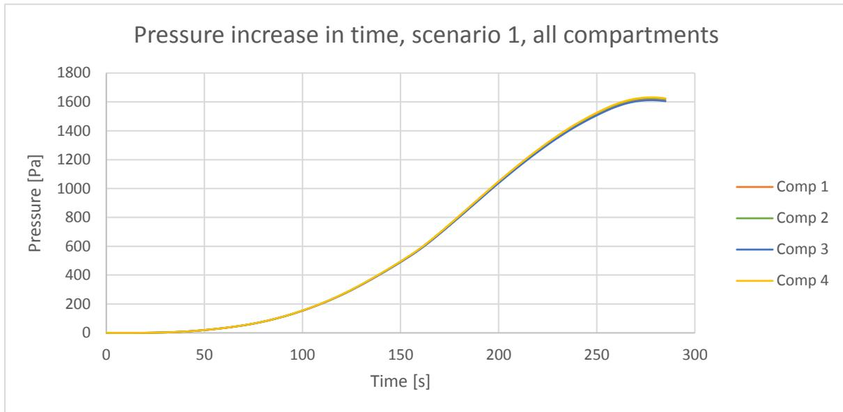
Figure 14 - Pressure increase in different compartments, scenario 1
