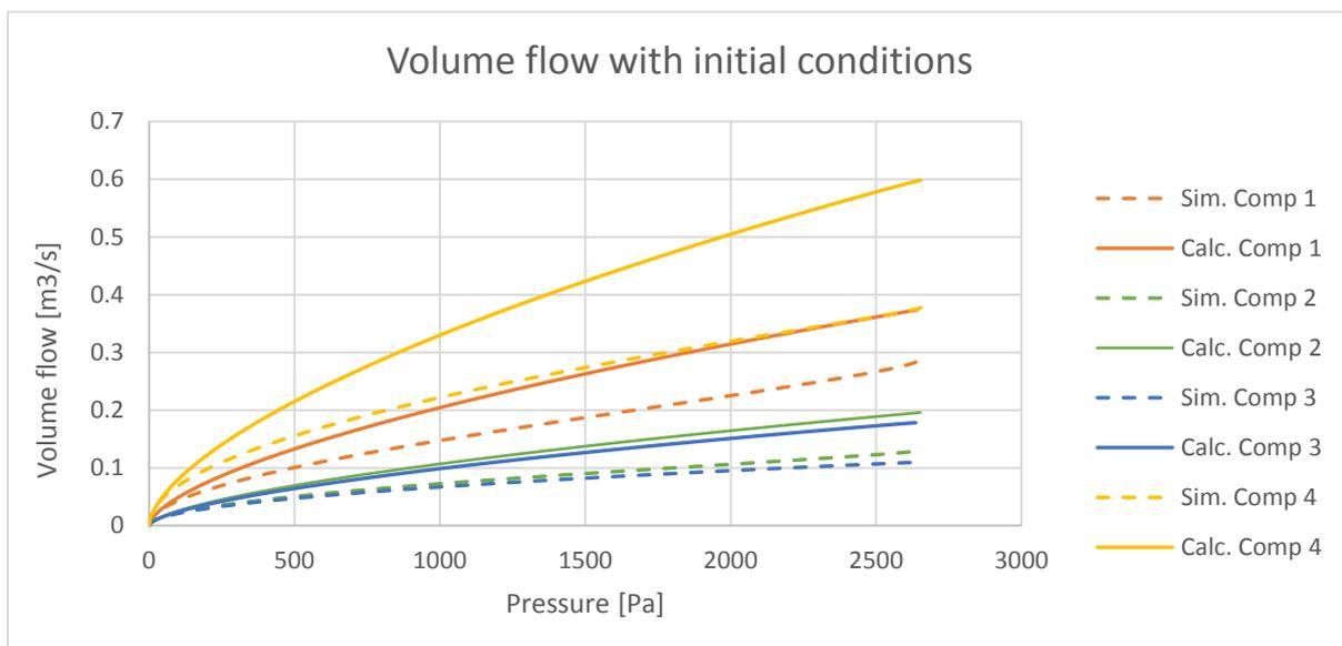
Figure 8 - Volume flow with constant openings as calculated
