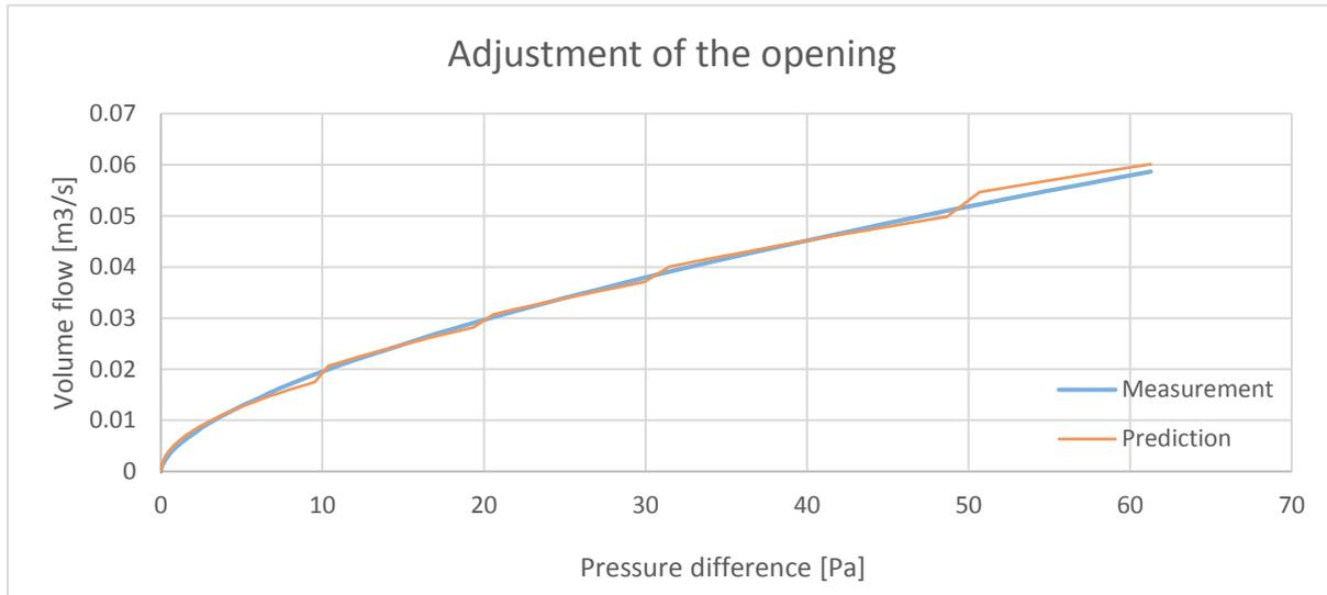
Figure 9 - Prediction of the volume flow by changing the opening for small pressure intervals
