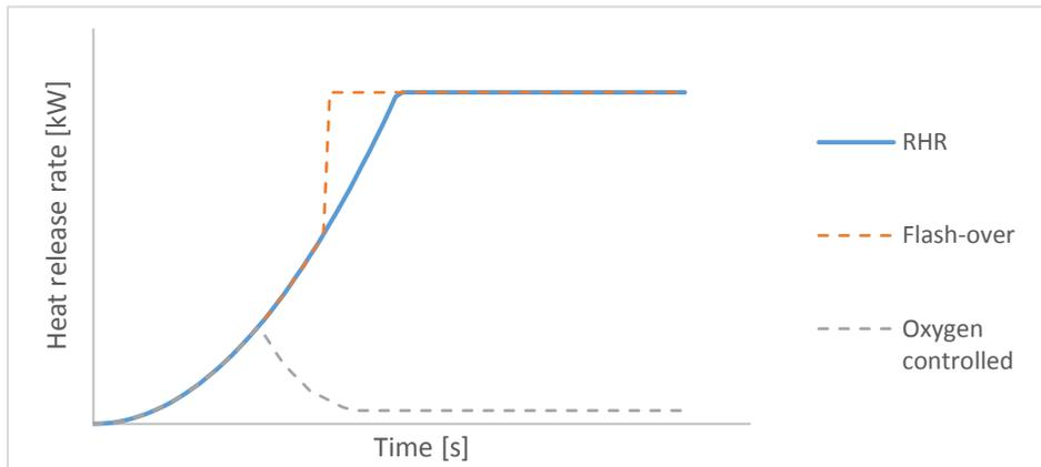
Figure 7 - Heat release rate according to  $t^2$ -curve, after flash-over and oxygen controlled
