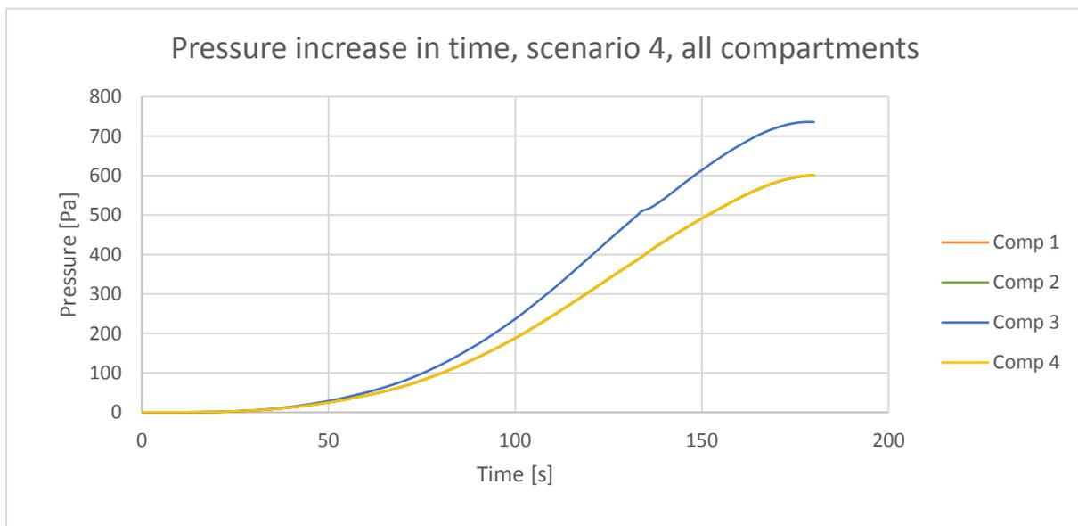
Figure 15 - Pressure increase in different compartments, scenario 4
