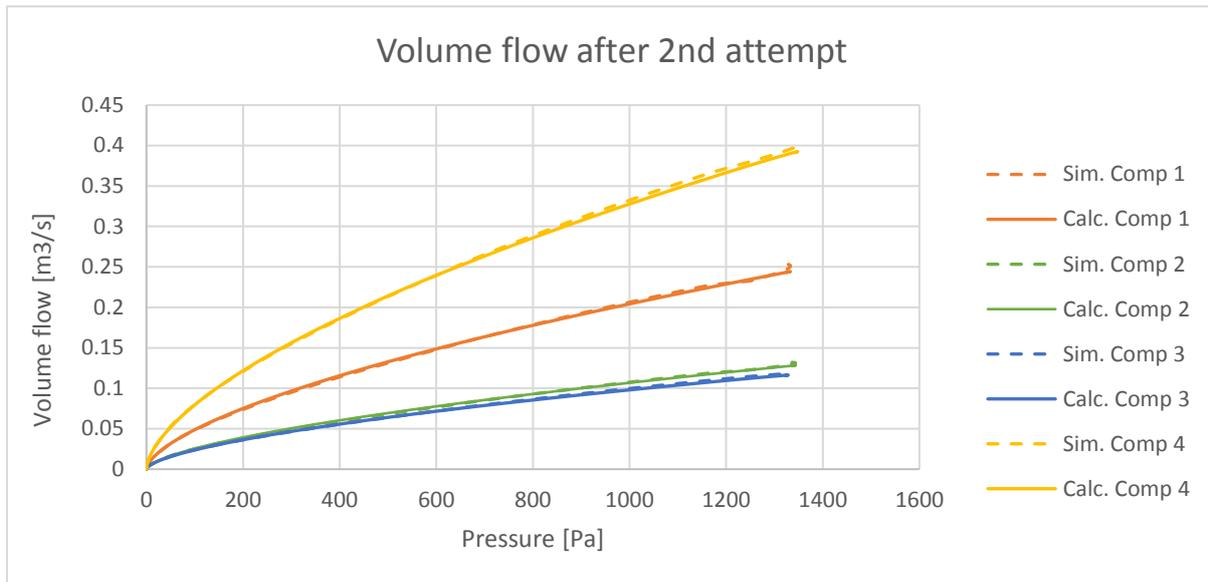
Figure 12 - Volume flow with variable openings, after 2nd attempt
