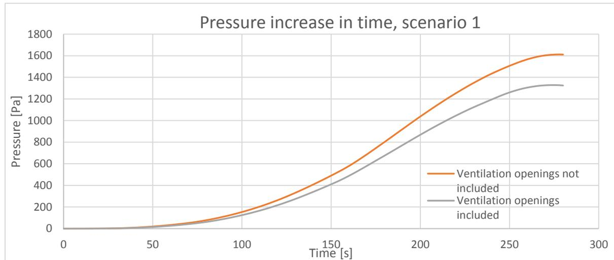
Figure 13 - Pressure increase in time, till maximum pressure is reached
