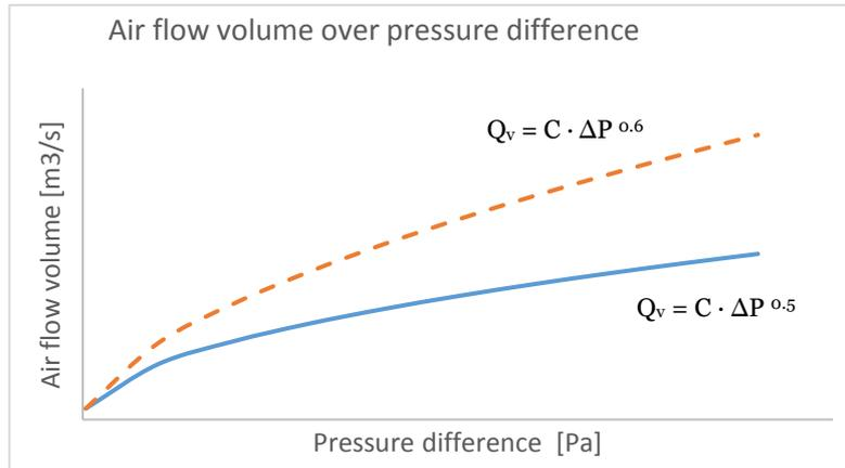
Figure 3 - Difference in air flow volume with different flow exponents
