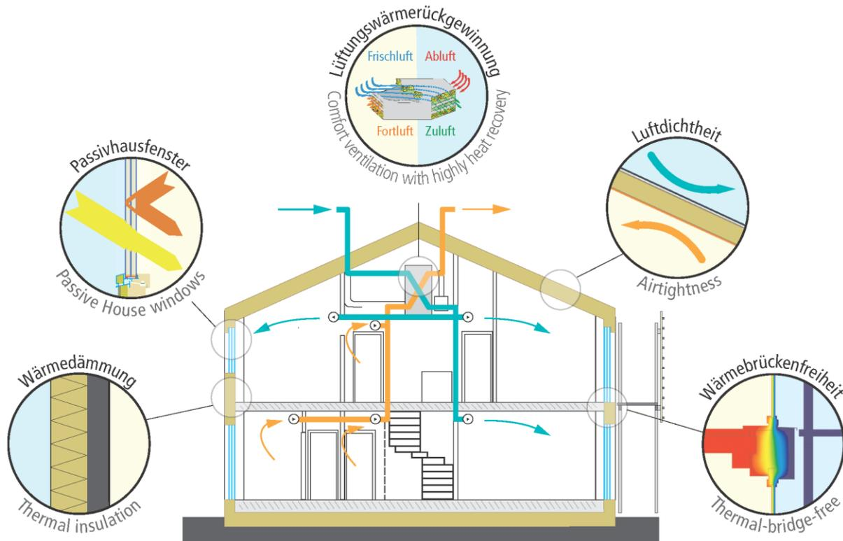
Figure 2 - Typical passive house solutions, source: (Passive House Institute, 2016)
