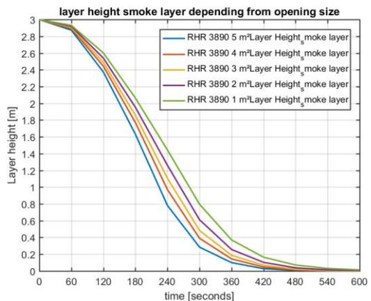
Figure 5 - smoke layer height in room 2 depending from opening size
