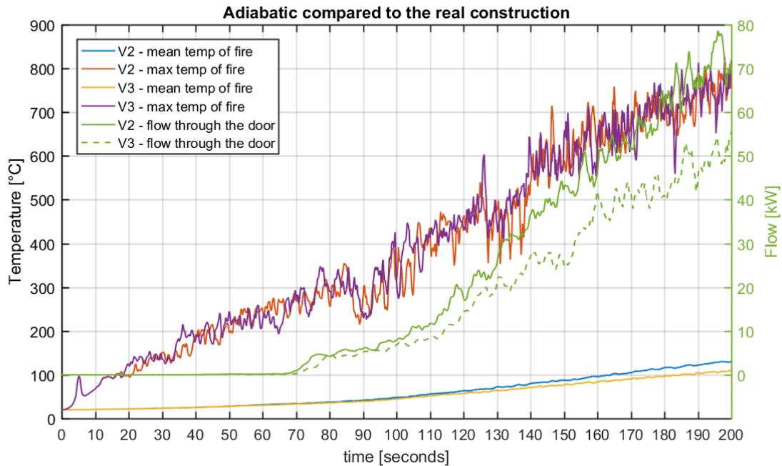
Figure 12 - Temperature of the in room 1 and the energy of the flow through the door in between
