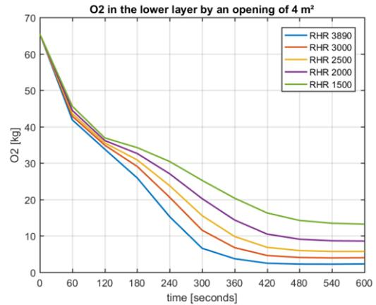
Figure 7 - O2 in the lower layer by an opening of 4 m<sup>2</sup>
