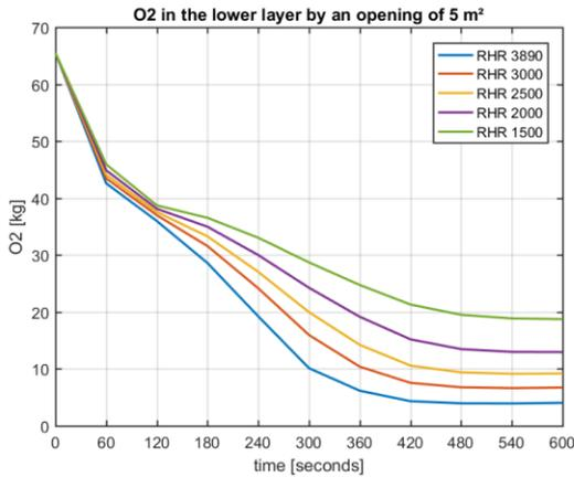
Figure 6 - O2 in lower layer by an opening of 5 m<sup>2</sup>
