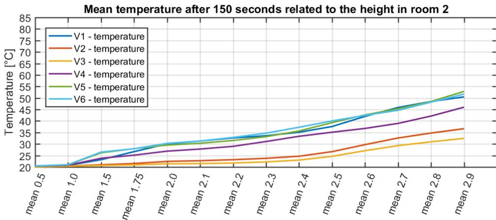
Figure 14 - Mean temperature after 150 seconds in room 2. The x-as represents the height of the thermocouple
