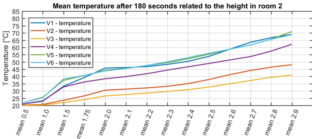
Figure 15 - Mean temperature after 180 seconds in room 2. The x-as represents the height of the thermocouple
