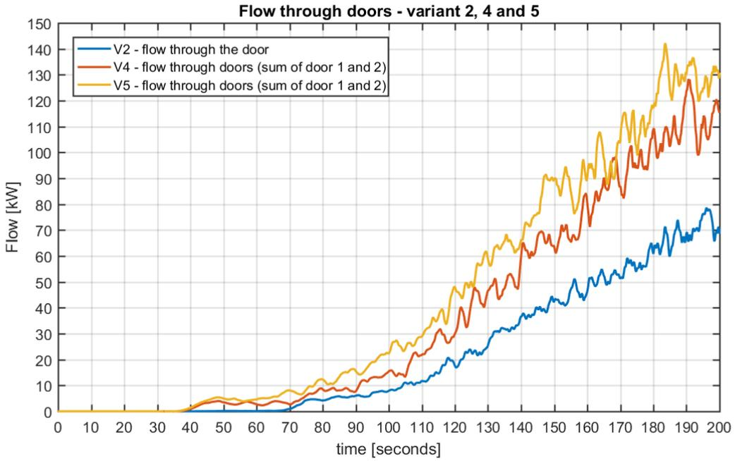
Figure 13 - Flow through the door(s) between room 1 and room 2 in kW for variant 2, 4 and 5.
