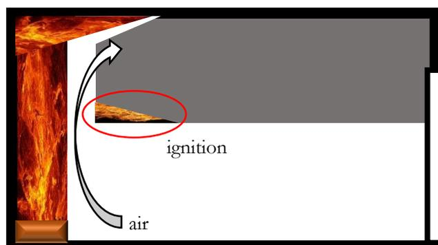
*Figure 1 – Schematic view of the observed effect by a firefighter. A part of the smoke layer, close to the flame, ignites.*
