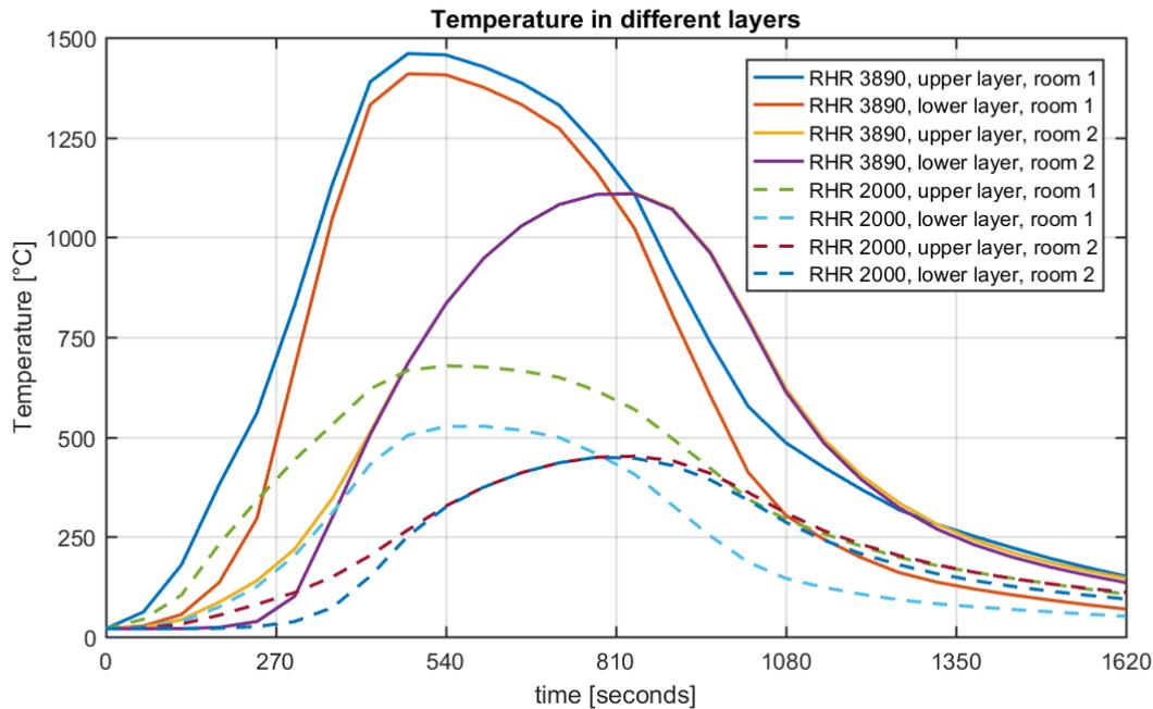
Figure 10 - Temperatures in the different layers. Comparison between a fire of 3,890 or 2,000 kW
