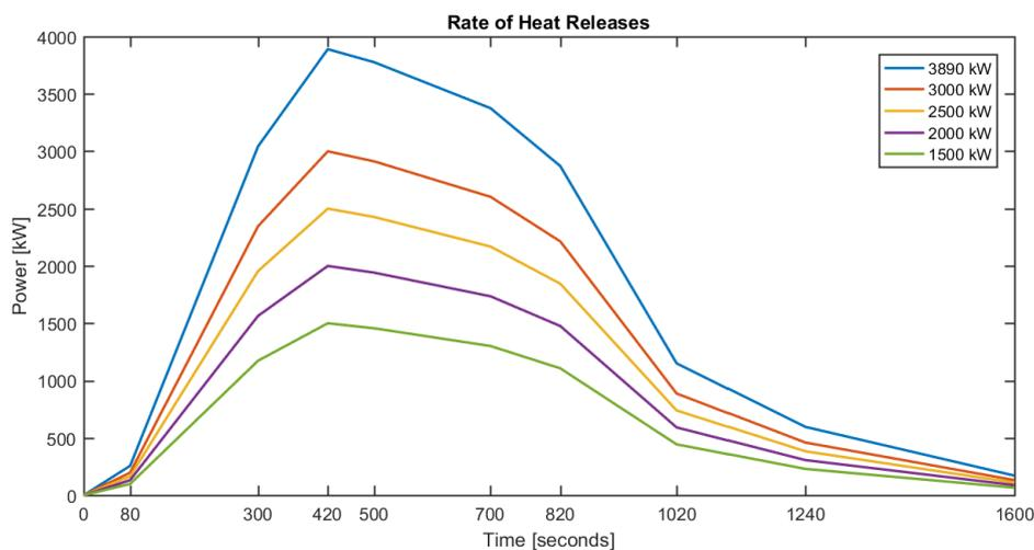
Figure 3 - Rate of Heat Release of the investigated woodpiles.
