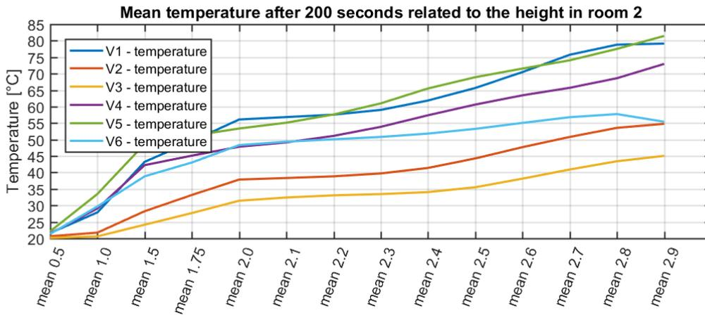
Figure 16 - Mean temperature after 200 seconds in room 2. The x-as represents the height of the thermocouple
