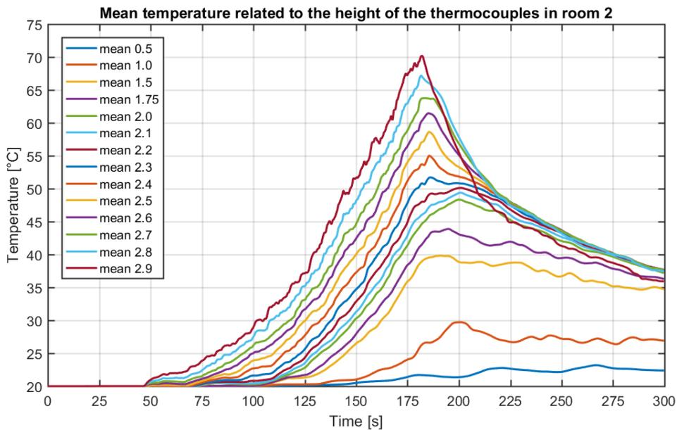
Figure 17 - Mean temperature over the height of the room related over the total depth of the room
