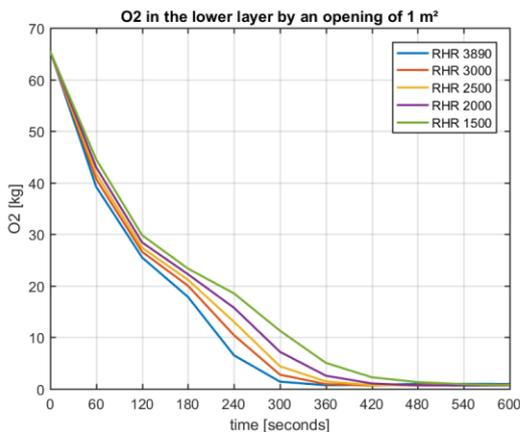
Figure 4 - O2 in the lower layer by an opening of 1 m<sup>2</sup>
