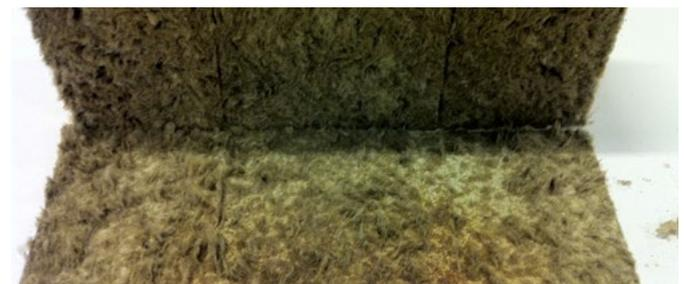
Figure 3.15: SWR sample after being exposed to 250 °C
