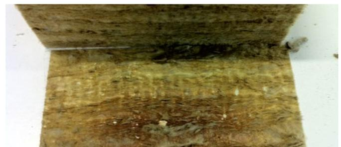
Figure 3.19: SWW sample after being exposed to 250 °C
