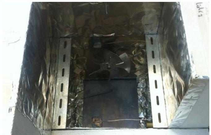
Figure 2.4: Rails to support the sample tray's
