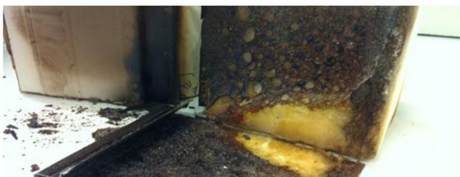
Figure 3.4: PUR sample with joint after being exposed to 350 °C
