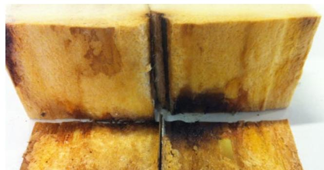
Figure 3.10: PIR sample with joint after being exposed to 350 °C
