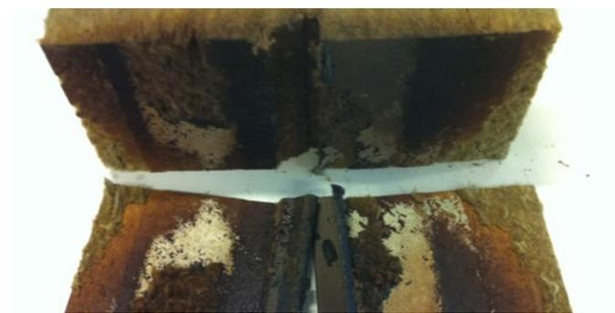
Figure 3.16: SWR sample with joint after being exposed to 350 °C
