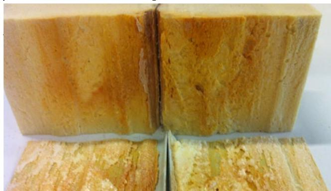
Figure 3.9: PIR sample with joint after being exposed to 250 °C
