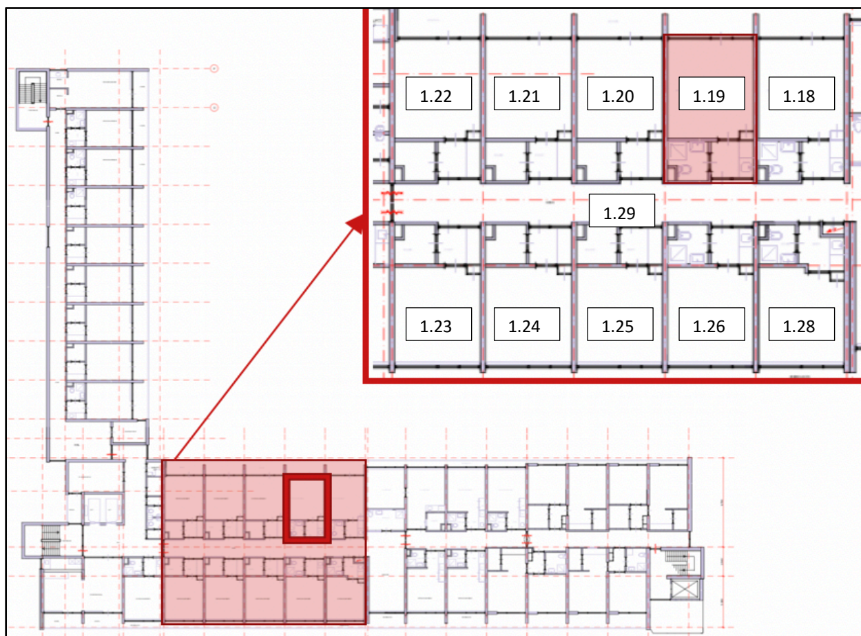
Figure 5 Floorplan first floor of the Schuylenburcht complex, room of fire origin is highlighted [20]
