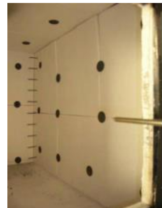
Figure 2: An example of a thermocouple tree with temperature sensors.
