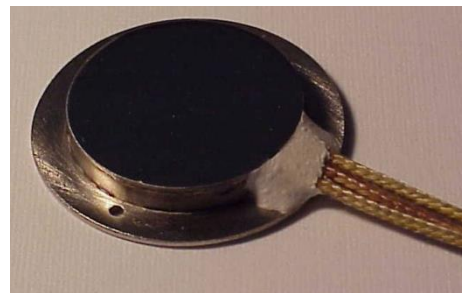
Figure 4: An example of the used heat flux sensor on the façade.
