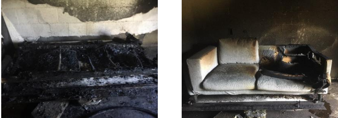
Figure 7: sofa after experiments for scenario 18 (left) and 16 (right), clear differences are observable relating to combusted mass.
